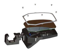
**Mirror Replacement** | To replace the convex mirror, first remove the six-M4 bolts, followed by the bezel, then carefully remove the convex mirror. Make sure to clean out any debris in the mirror cavity before replacing the mirror. To install new mirror follow the previous steps in reverse.
