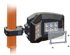
**Lens Replacement** | To replace either of the lenses, first remove the four-M4 bolts, followed by the bezel, then carefully remove the lens. Make sure to clean out any debris from the LED cavity and make sure that the O-ring is clean and clear of debris as well. To install new lens follow the previous steps in reverse. Tighten bolts incrementally in a diagonal pattern to reduce chance of glass breaking. Torque spec.: 70 in/lb.
