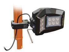
**Step 5** | Adjust mirror/light to preferred angle and then tighten adjustment screw to desired firmness. *Do not exceed 60 in/lb.*
