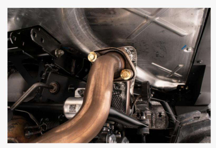
2. Using a spring puller, rope, or wire remove the (2) springs on either side of the original silencer. Take caution not to let the silencer fall of the machine and damage other components.
