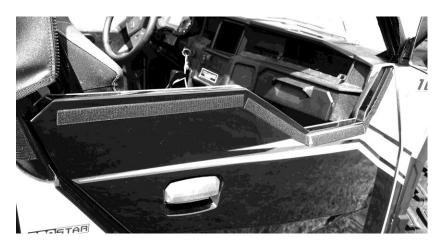
8. After all the Velcro is in place take the door and place it on the vehicle. The following series of photos show how it should look after being installed.
