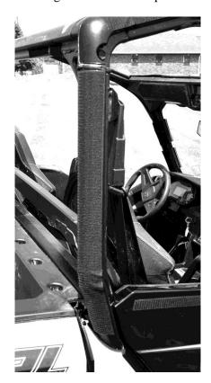
7. Now move to the top of the door. Starting at the front place the 12" along the top of the door on the outside. Then follow the different angles of the door and place two 10" strips then a 12" strip. As shown in the photobelow.
