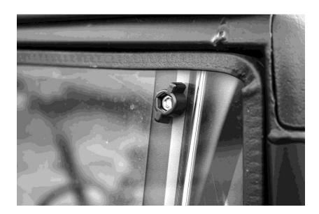
4. Next take the Metal brackets and bolt them to the Rear Window from the inside using the supplied 1" bolts washer and thumbnut as shown in the picture below.
