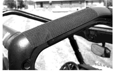
7. Next place the 20" strip down the back of the cage as shown in the photo below.
