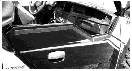
9. After all the Velcro is in place take the door and place it on the vehicle. The following series of photos show how it should look after being installed.
