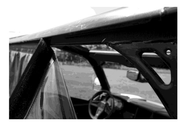
11. After the adhesive Velcro strips have been installed along the top and down the sides you can now place your rear window in the frame. Lastly mark where the bottom of the rear window sits on the vehicle and place the 48" adhesive strip flat on the vehicle so the bottom of the rear window pulls into the cab and attaches downwards.
