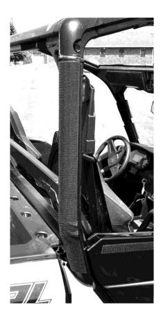
8. Now move to the top of the door. Starting at the front place the 12" along the top of the door on the outside. Then follow the different angles of the door and place two 10" strips then a 12" strip. As shown in the photo below.
