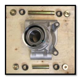
c. Insert the bushings, pivot tubes, and pivot caps into the collars of the **rear right backing plate (89X-R). NOTE**: We recommend applying good water-resistant grease to the bushings and especially the pivot tube. This will help prevent excessive friction & wear plus add longevity to the life of the bushings and pivot tube.
