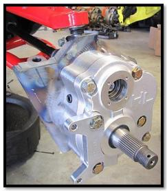
d. Loosely fasten the all four bolts with **1/2" flat washers** and **1/2" lock nuts**. Recheck all parts that were used and make sure everything fits correctly, and then go ahead and fasten all bolts. (3/4) [105 ft lbs]
