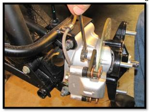
b. Remove the caliper from the rear hub. Leave the brake hose attached to the caliper and hang the calipers out of the way. Take precautions to ensure the brake hose isn't stretched or pinched.
