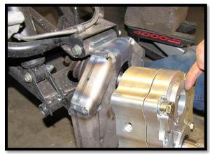
d. Loosely fasten the all four bolts with ½" flat washers and ½" lock nuts. Recheck all parts that were used and make sure everything fits correctly, and then go ahead and tighten and torque all bolts. (3/4) [105 ft lbs]
