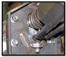
e. Install the tie rod end into the backing plate tie rod mount bracket. Fasten the tie rod end with the factory hardware. (18mm) [90 ft lbs]
