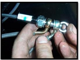
c. Install the new longer brake line **PGLC-BRAKELINE** to the banjo bolt. Run the line back through the frame and to the (PA) side hub.
