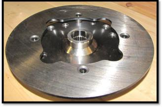
g. Apply **LOCTITE (RED)** to (4) **3/8-16 x 1" button head bolts**. Insert the screws through the rotor, the spacers, and then into the hub. Tighten and torque. (7/32) [45 ft lbs]
