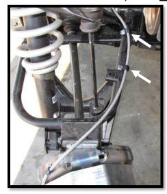
g. Next, slide a **p-clamp** over the brake line. Secure it to the rear backing plate using a **5mm x 20mm bolt** through the clamp and backing plate, followed by a **5mm washer** and **5mm lock nut**.
