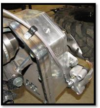
h. Once the lines are secured, make sure there is no binding, pinching, or in contact of moving parts.
