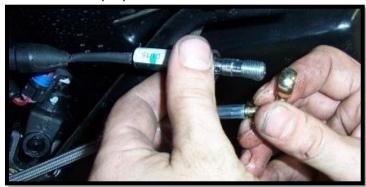
d. Use the existing factory (PA) side brake line and install it to the banjo bolt. This is replacing the factory (DR) side brake line.
