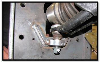
c. Insert the drive shaft into the backing plate. Then place the upper ball joint into the upper ball joint mount bracket. Fasten it with the factory hardware. (15mm) [50 ft lbs]
