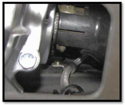
f. If you are <u>using factory upper arms</u>, you can re-secure the brake lines using the factory p-clamps or the new supplied **p-clamps**. Secure them to the upper arms using **5mm x 16mm bolts**, followed by **5mm washers** and **5mm lock nuts**. If you are <u>using aftermarket upper arms</u>, secure brake lines with **zip ties**.
