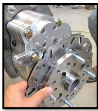
d. Slide on the supplied **30mm lock washer**, followed by the **30mm spindle castle nut**. (46mm) [**Min 120 ft lbs**] Tighten the castle nut further if needed to align grooves with holes in the spindle for the cotter pin. Install the supplied **cotter pin**. Both ends of the cotter pin must be folded.
