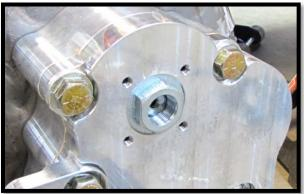
c. Align the portal box lid cap & gasket. Use the 1/4-20 x 3/4" screws and install to the portal box. [8 ft lbs]
