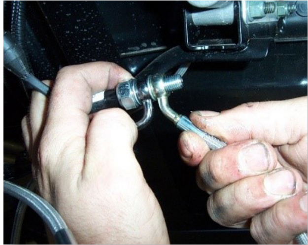
Route the line back through to the right front control arm.
