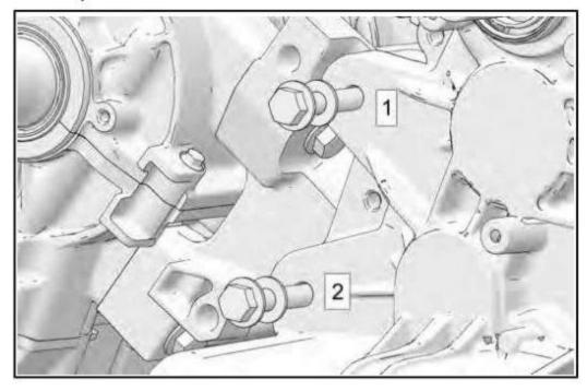
Torque right side mounting bolts to specification using the numbered sequence shown.
