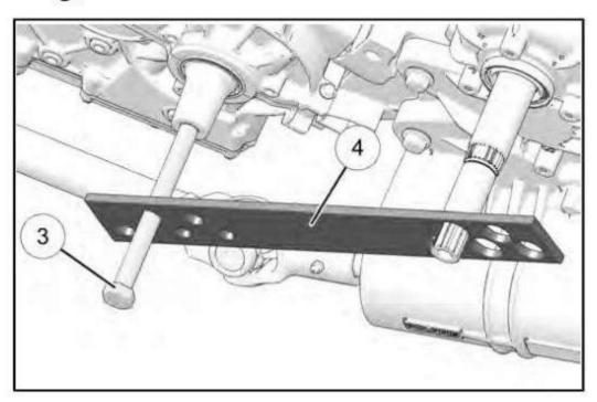
Loosen the two bolts retaining the transmission coupler bracket to the engine on the right side.
