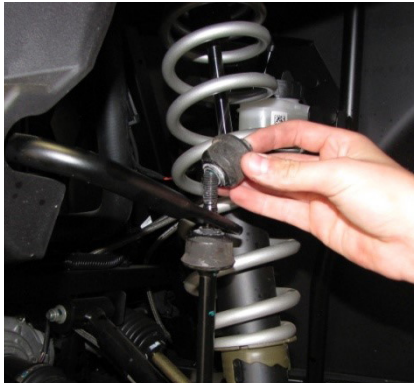
Disconnect the upper end of the sway bar link.
