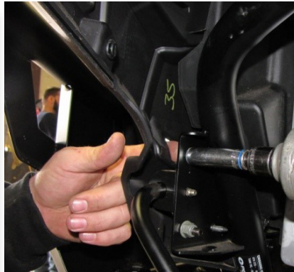
Remove the lock nuts and bolts that attach the bar to the front frame.
