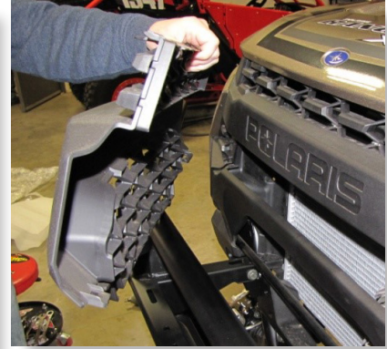
Remove the front grill insert to gain access to the sway bar.
