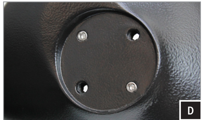
D. Find the best orientation for the speaker on your bar and screw in the Set Screws in the OPPOSITE holes of where the clamp will install into using a 4mm allen wrench
