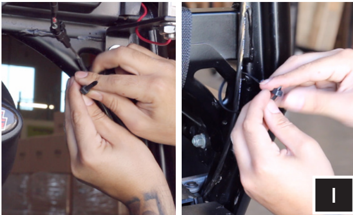
I. Using the provided zip ties tie down speaker wire alongside the roll cage.
