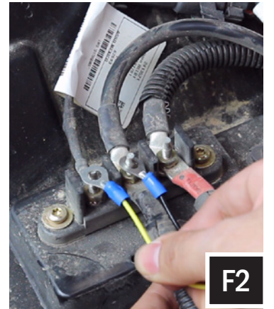
F. At the Bus Bar terminal located under the hood, unscrew the nut on the second position terminal and attach the black Ground wire. Refasten the nut. Then connect the yellow Power wire to either the constant terminal (F1) or the accessory terminal (F2). Refasten the nut.
