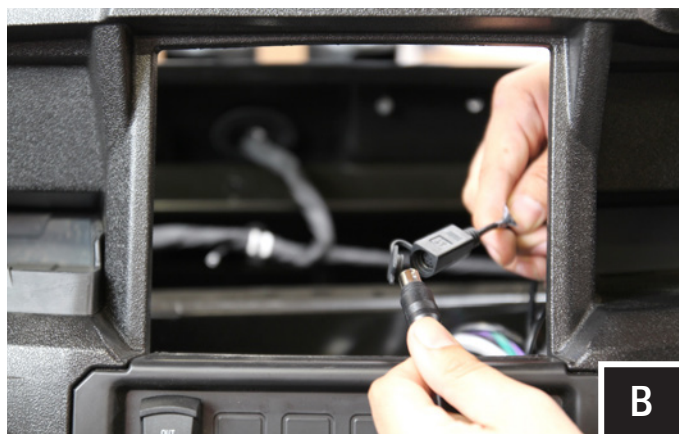
B. Connect MRB3 controller to the MRB3 Brain and secure cables.
