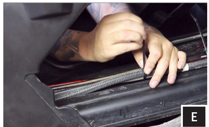
E. Zip tie all cables to the factory cabling along the center column away from the drive shaft.
