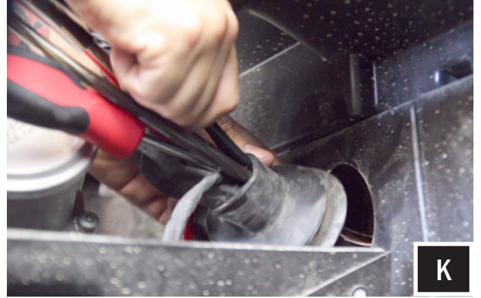
K. Unwrap the tape from rubber grommet and feed the power/ground wire for the Amp through the grommet as well as the rear speaker harness H1151.
