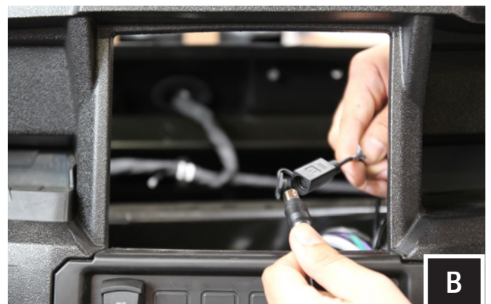
B. Connect MRB3 controller to the MRB3 Brain and secure cables.
