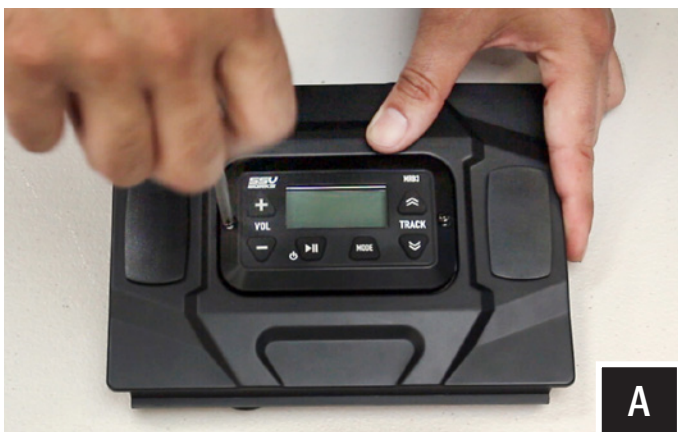
A. With a #2 Phillips screw driver, secure the MRB3 controller to the dash kit with the 2 screws supplied in the MRB3 box.
