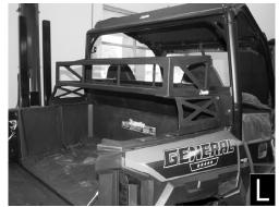
**Step 15:** Place P4 through P5. Then place through holes of cargo rack and bed mount. Install bolt with a P5 and P8. (Figure M)
